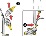
3 Remove clear bin and cyclone top, by lifting up until it releases. Then gently pull off from ball socket.
