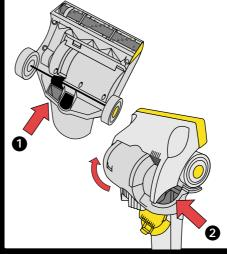
Turn machine upside down. Remove soleplate. Raise inspection flap 1 and look down through aperture. If you cannot see daylight, remove any blockage with a stiff wire.
