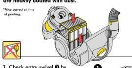
1. Check entry swivel 1 by pressing yellow buttons & pulling out hose. Clear any debris.
