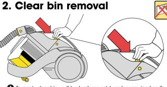
1 To empty clear bin, pull back release catch under carrying handle and raise top of machine.
