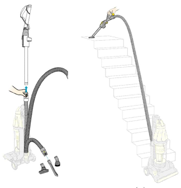
Press the wand release button and remove the wand. Fit one of the tools directly on to the end of the hose. Use tools for confined spaces such as car cleaning.
