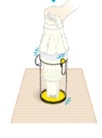
To reassemble the clear bin, place on the floor with the clear bin base closed.
