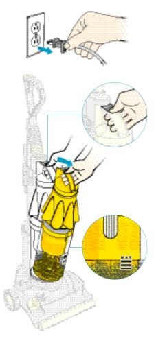
To ensure your machine continues to clean effectively, the clear bin must be emptied when the dust reaches the MAX mark.
