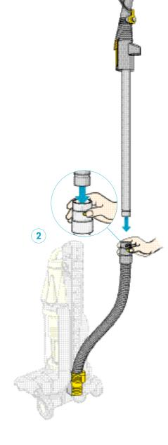
2 Pressing the wand release button, slide the wand down inside the hose.
