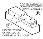
The DSA230 and the DSA250 loudspeakers differ in length. They are both secured in the their packaging by similar parts. The longer DSA250 requires two cardboard top pads (F) and the shorter DSA230 requires only one.
