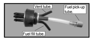
Carefully use a lighter or heat gun to permenently set the angle of the vent tube.
