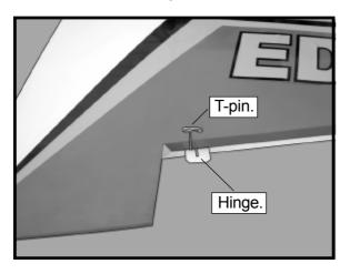
$\square$  3) Slide the aileron on the wing panel until there is only a slight gap. The hinge is now centered on the wing panel and aileron. Remove the T-pins and snug the aileron against the wing panel. A gap of 1/64" or less should be maintained between the wing panel and aileron.
