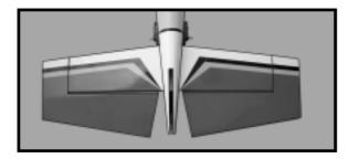
□ 8) After the epoxy has fully cured, remove the masking tape or T-pins used to hold the stabilizer in place. Carefully inspect the glue joints. Use more epoxy to fill in any gaps that may exist that were not filled previously and clean up the excess using a paper towel and rubbing alcohol.
