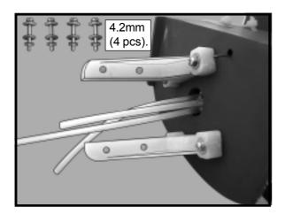
□ 5) Bolt the engine to the engine mount using the four machine screws. Double cheek that all the screws are tight before proceeding.
