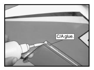
$\Box$  5) Turn the wing panel over and deflect the aileron in the opposite direction from the opposite side. Apply thin C/A glue to each hinge, making sure that the C/A penetrates into both the aileron and wing panel.
