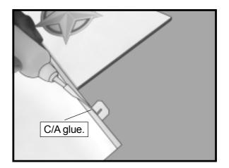
□ 4)Deflect the rudder and completely saturate each hinge with thin C/A glue. The rudder front surface should lightly contact the vertical fin during this procedure. Ideally, when the hinges are glued in place, a 1/64" gap or less will be maintained throughout the lengh of the rudder to the fuselage panel hinge line.
