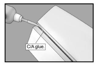
$\square$  6) Using C/A remover/debonder and a paper towel, remove any excess C/A glue that may have accumulated on the wing or in the aileron hinge area.
