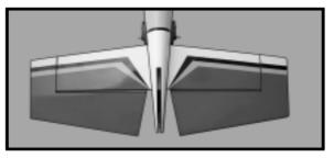
$\Box$  4) With the stabilizer held firmly in place, use a pen and draw lines onto the stabilizer where it and the fuselage sides meet. Do this on both the right and left sides and top and bottom of the stabilizer.
