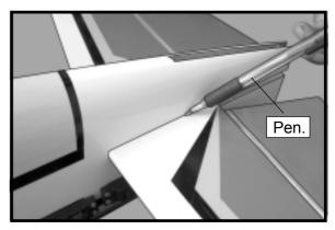
$\Box$  5) Remove the stabilizer. Using the lines you just drew as a guide, carefully remove the covering from between them using a modeling knife.
