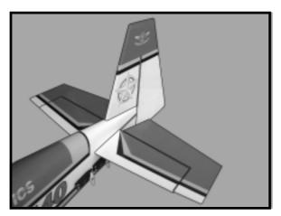
$\Box$  3) While holding the vertical stabilizer firmly in place, use a pen and draw a line on each side of the vertical stabilizer where it meets the top of the fuselage.
