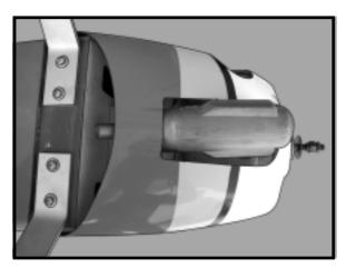
$\Box$  3) Slide the cowl back over the engine and secure it in place using six 3mm x 10mm wood screws. See picture below.
