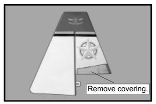
When cutting through the covering to remove it, cut with only enough pressure to only cut through the covering itself. Cutting into the balsa structure may weaken it.
