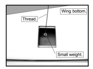
Attach the string to the servo lead and carefully thread it though the wing. Once you have thread the lead throught the wing, remove the string so it can use for the other servo lead. Tape the servo lead to the wing to prevent it from falling back into the wing.
