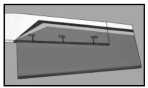
□ 4)Deflect the elevator and completely saturate each hinge with thin C/A glue. The elevators front surface should lightly contact the horizontal stabilizer during this procedure. Ideally, when the hinges are glued in place, a 1/64" gap or less will be maintained throughout the lengh of the elevator to the horizontal stabilizer panel hinge line.
