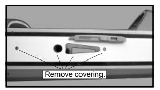
Attach the aluminium tube into fuselage.
