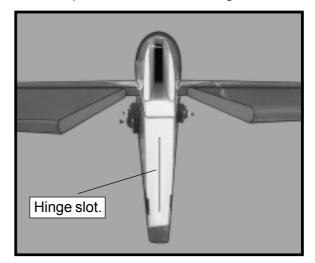
□ 2) Slide the vertical stabilizer into the slot in the top of the fuselage. The rear edge of the stabilizer should be flush with the rear edge of the fuselage and the lower rudder hinge should engage the precut hinge slot in the lower fuselage. The bottom edge of the stabilizer should also be firmly pushed against the top of the horizontal stabilizer.
