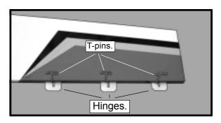
□ 3) Slide the elevator on the horizontal stabilizer panel until there is only a slight gap. The hinge is now centered on the horizontal stabilizer panel and elevator. Remove the T-pins and snug the elevator against the horizontal stabilizer panel. A gap of 1/64" or less should be maintained between the horizontal stabilizer panel and elevator.
