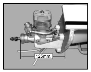
$\Box$  2) Place your engine onto the engine mount. Adjust the engine is centered of the edges of the engine case.
