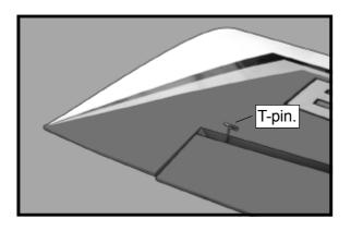
$\Box$  4)Deflect the aileron and completely saturate each hinge with thin C/A glue. The ailerons front surface should lightly contact the wing during this procedure. Ideally, when the hinges are glued in place, a 1/64" gap or less will be maintained throughout the lengh of the aileron to the wing panel hinge line.
