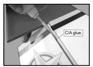
$\Box$  5) Turn the vertical fin panel over and deflect the rudder in the opposite direction from the opposite side. Apply thin C/A glue to each hinge, making sure that the C/A penetrates into the rudder and fuselage panel.
