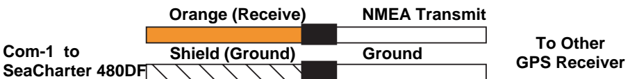
Com-1 wiring to receive NMEA position information from some other GPS receiver.
