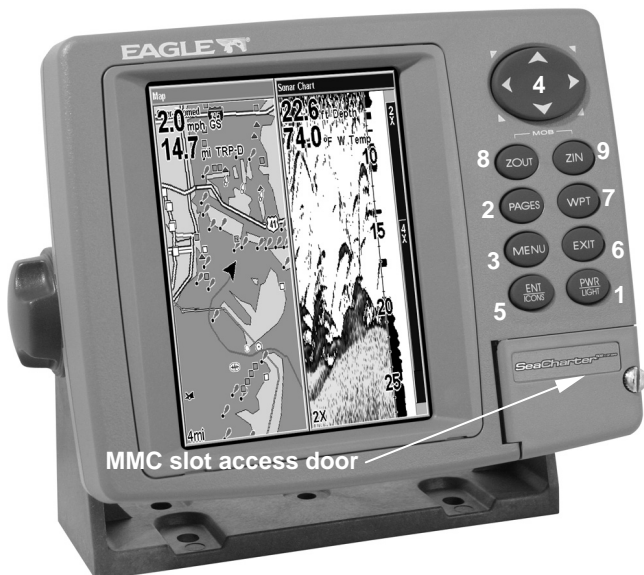
SeaCharter 502cDF iGPS unit showing map with sonar page, keyboard and access door for MMC cards.
