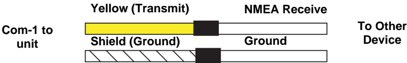
Com-1 wiring to transmit NMEA position information to another NMEA-compatible device.
