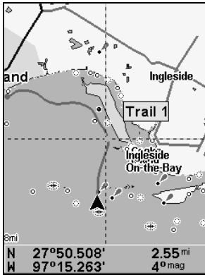
Trail selected with map cursor (left). The box at the bottom of the screen shows distance and bearing from current position to the selected point on the trail. The Edit Trail menu (right).
