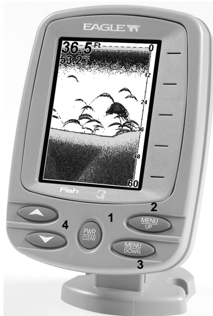
FishEasy 320C Sonar, front view, showing screen and keyboard.
