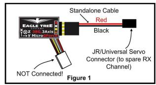
IMPORTANT: Ensure that you connect the Standalone Cable with the correct polarity, or the G-Sensor could be damaged, voiding the warranty! Note that in Standalone Mode, the 4 wire cable built into the G-Sensor must NOT be connected to anything!
