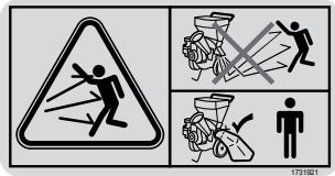
Decal - Danger, Thrown Objects, Do Not Operate Without Collection Bag, CE Models
