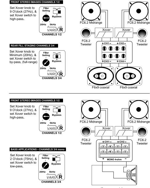
Kompressor tube in mono application (4 ohms minimum).
