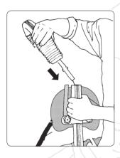
Fig. 2 Let the tube slide into the back support bar and pull over the bellows.
