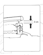
Fig. 5 Leave a gap of approx. 2 cm (1 inch) between the camera and the support arm.
