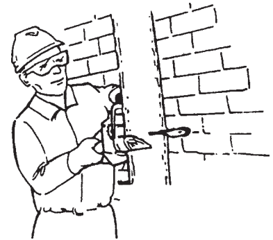
KICK GUARD® ALLOWS KICK-BACK FREE CUTTING NEAR MASONRY, FENCES, ETC.
