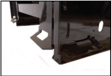
The chipper has two mounts, so it can be set to feed in front or to the curb side
