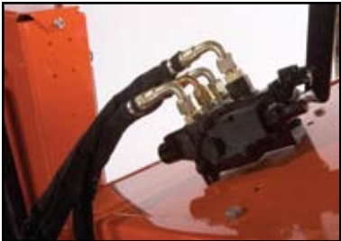
The four-position valve easily controls the hydraulic feed roller
