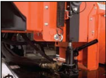
Built-in hydraulic jack makes feed roller maintenance quick and easy.
