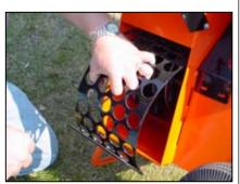
The Discharge Screen is easily removable making the change from screen to screen a breeze.
