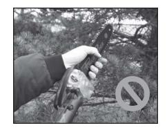
After shutting off the engine or motor, keep your fingers and body away from the cutting attachment until all movement has stopped. Saw chain or blade will coast to a stop after releasing the throttle.
