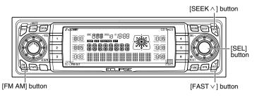
First, press the [FM AM] button to start tuner operation.
