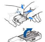
Carefully lift up the cover of the battery (3).
