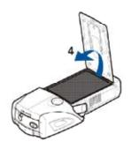
Remove the battery from the compartment (4).
