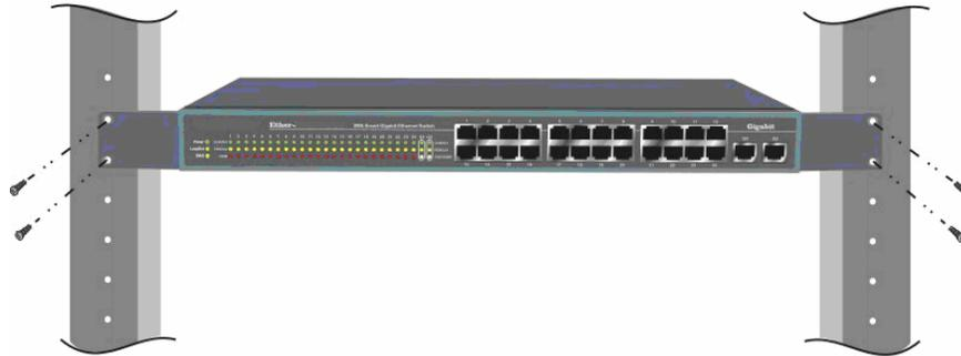
**Fig. 3-2 Attaching the Switch to a 19-inch rack**
