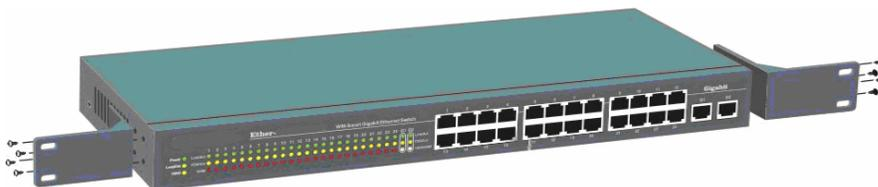
**Fig. 3-1 Fastening the brackets on the switch**
