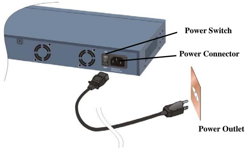
Fig 3-13 Connecting the Switch to power outlet
