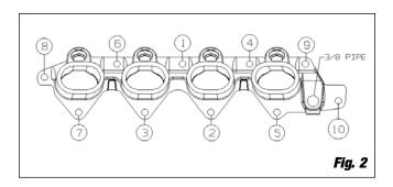
Install fuel injectors, stock fuel rail spacers and fuel rail. Each injector should be able to rotate freely after the fuel rail holdown bolts are fully tightened.
