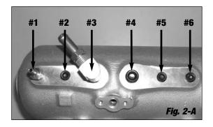
Install the vacuum fittings into the top of the Performer X intake manifold (See Fig. 2-B).
