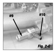
2. Remove Idle air control motor from factory intake manifold and install onto the Performer X intake manifold
