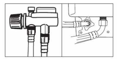
Your dishwasher comes equipped with a 'quick-connect' assembly (includes inlet and drain hose). The faucet adapter must be installed on the faucet before you can connect the dishwasher. This adapter is included inside your dishwasher.
