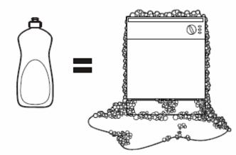
Using a detergent that is not specifically designed for dishwashers will cause the dishwasher to fill with suds. During operation, these suds will spill out of the dishwasher vents.
