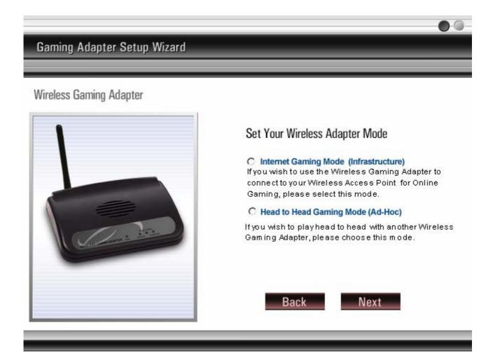
6. In the "Internet Gaming Mode (Infrastructure)", the Wireless Gaming Adapter has to connect to an access point before going to the Internet. You can select "Scan For Your Local Wireless Network" to let the Wireless Gaming Adapter automatically scan for an available access point and jump to step 7. If already know the SSID of the available access point, you also can select "Assign Your Wireless Network Manually", enter the SSID of the access point and jump to step 10.
