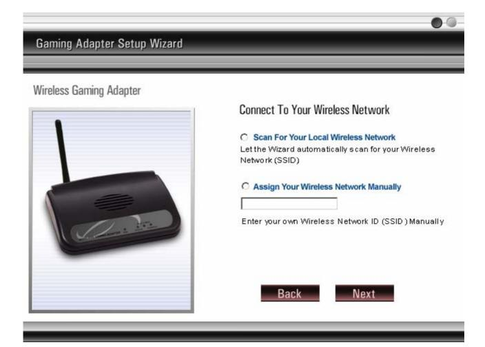
7. The Wireless Gaming Adapter automatically scans for all available access points and lists their SSID. If the Wireless Gaming Adapter does not find any access point, click "Scan" to let it search again. You can select one access point and click "Next". Jump to step 10.
