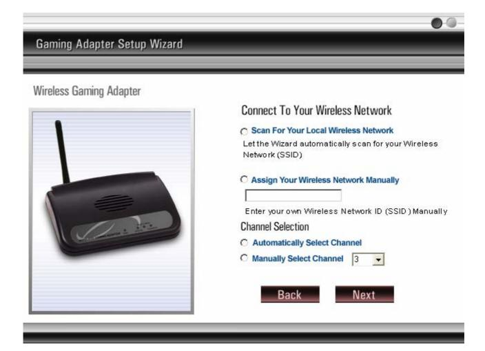
9. The Wireless Gaming Adapter automatically scans for all available wireless devices, including Wireless Gaming Adapters, with Ad Hoc mode and lists their SSID. If the Wireless Gaming Adapter does not find any wireless device, click "Scan" to let it search again. You can select one wireless device you want to connect to and click "Next".
