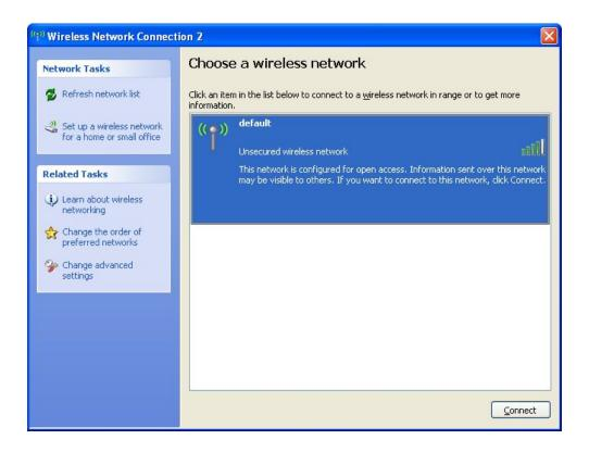
8. If the access point is protected by encryption, you have to input its security key or passphrase here. It must match the encryption setting on the access point.
