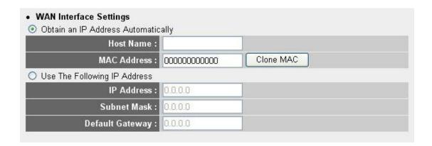
Please select the type of how you obtain IP address from your service provider here. You can choose 'Obtain an IP address automatically' (equal to DHCP, please refer to 'Cable Modem' section above), or 'Use the following IP address' (equal to static IP address, please refer to 'PPPoE xDSL' section above).
