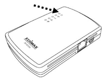
Note: The 'Power' LED is lit in green color when the battery is charged completely if router is activated before charged.
