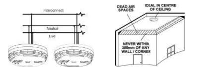
Be very careful about correctly wiring the alarms as mixing Live and Neutral will blow/damage interconnected alarms.
