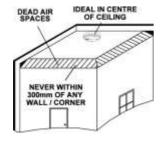
Alarms should be placed in accordance with the general guidelines shown in the diagram above. These recommendations are based on the problem of areas of "dead air" close to corners of rooms and apexes of ceilings, which could result in the prevention of smoke reaching the smoke detector
