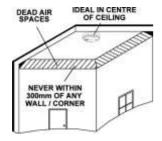
Place the mounting plate on the ceiling/wall and mark the screw holes. Drill with a suitable drill bit, insert the screw plugs and screw the plate into position. Simply slide the alarm into position on the mounting plate (this also activates the battery connection).
