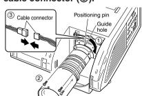
(When the lens being attached is the AH-45401 (EIP-4500 standard lens) or AH-51401 (EIP-5000 standard lens))
