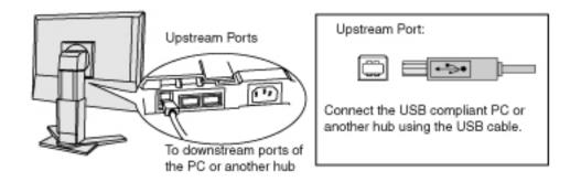
After connecting the USB cable, the USB function can be set up automatically.
