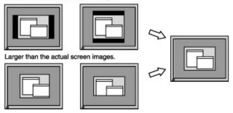
4.Adjust the output signal range (Dynamic Range) of the signal. => 2 Use the <<u>Range Adjustment</u>> of <Screen> menu.
