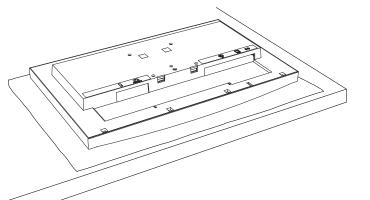
${\bf 2}\,$  Put the insertion part of the stand in the slot of the monitor.
