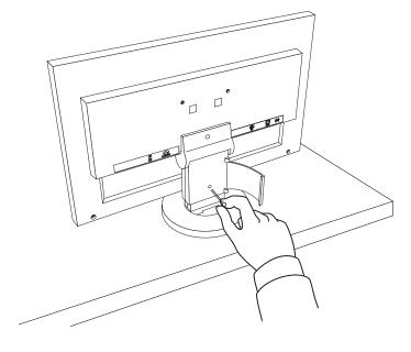
**3** Lay the LCD monitor on a soft cloth spread over on a stable surface with the panel surface facing down.
