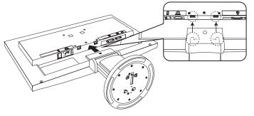
**3** Prepare a screwdriver. Press the upper part of the stand against the unit and tighten the screw with the screwdriver to fix the stand to the unit.
