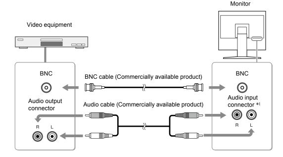
\*1 The monitor is equipped with a single audio input connector to connect for either a PC or visual equipment. Regardless of the input device selected, the monitor will output sound.
