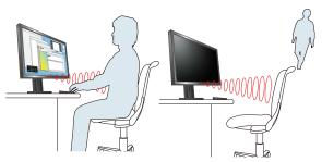
EcoView Sense automatically signals the screen to activate and stay on, or switch to power save mode by detecting whether the user is present or not.
