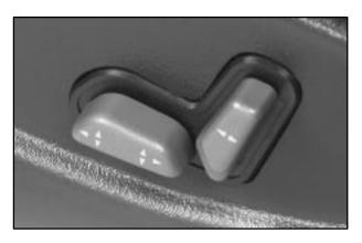
**Horizontal Control:** Raise or lower the front of the seat by raising or lowering the forward edge of the control.
