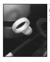
The engine oil dipstick handle on the "VORTEC" 4300 V6 engine is a yellow ring.
