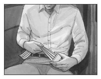
Each jump seat has a lap belt with no retractor. To make the belt longer, tilt the latch plate and pull it along the belt.
