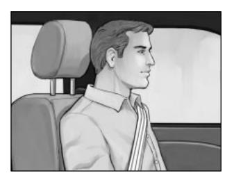
Head restraints are fixed on some models and adjustable on others. Slide an adjustable head restraint up or down so that the top of the restraint is closest to the top of your head. This position reduces the chance of a neck injury in a crash.
