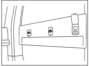
Anchor points for the top strap in a regular or extended cab are located behind the front seat.
