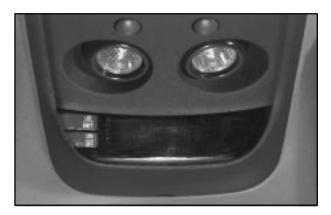
The outside air temperature and the compass are displayed at the front of the overhead console. The control buttons are located to the left of the display. Turn the display on or off by pressing the ON/OFF button. Display the temperature in either degrees Fahrenheit (English) or Celsius (metric) by pressing the US/MET button.
