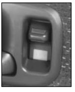
To unlock the door, slide the lever on the door up. You will see a red area on the lever.
