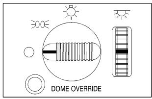
The control on the driver's side of the instrument panel operates the exterior lamps
