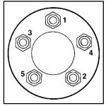
10. Use the wrench to tighten the wheel nuts firmly in a crisscross sequence as shown.
