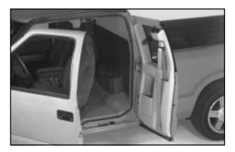
Your vehicle may be equipped with a side access panel for convenience in loading and unloading cargo.
