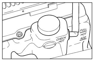
The coolant level should beat least up to the ADD mark. If it isn't, you may have a leak at the pressure cap or in the radiator hoses, heater hoses, radiator, water pump or somewhere else in the cooling system.
