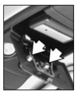
The pegs inside the compartment door are used to make sure the button on the compartment door will contact the control button on the garage door opener.
