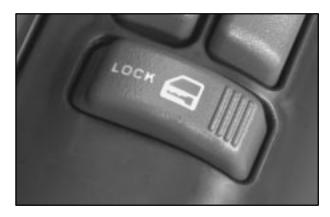
If your vehicle has power door locks, the switch is located on the armrest. Remove the ignition key and press LOCK to lock all the doors at once.
