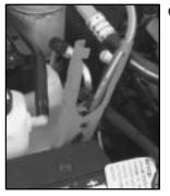
6. Connect the red positive (+) cable to the positive (+) terminal of the dead battery. Use a remote positive (+) terminal if the vehicle has one.
