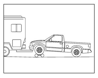
Your vehicle should not be towed with all four wheels on the ground. Your transmission has no provision for internal lubrication while being towed. To properly tow your vehicle, it should be placed on a platform trailer with all four wheels off the ground. Towing with all four wheels on the ground should be avoided.
