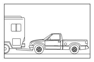
Your vehicle should not be towed with all four wheels on the ground. Your transmission has no provision for internal lubrication while being towed. To properly tow your vehicle, it should be placed on a platform trailer with all four wheels off the ground. Towing with all four wheels on the ground should be avoided.
