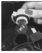
2. Twist the bulb socket counterclockwise to remove it from the headlamp assembly.
