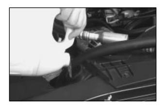
3. Fill the radiator with the proper DEX-COOL® coolant mixture, up to the base of the filler neck. See "Engine Coolant" in the Index for more information about the proper coolant mixture.
