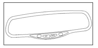
This mirror automatically changes to reduce glare from headlamps behind you. A photocell on the back of the mirror senses when it is becoming dark outside. Another photocell built into the mirror surface senses when headlamps are behind you.
