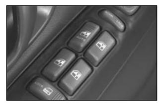
Press the side of the switch with the down arrow to lower the window. Press the side of the switch with the up arrow to raise the window.
