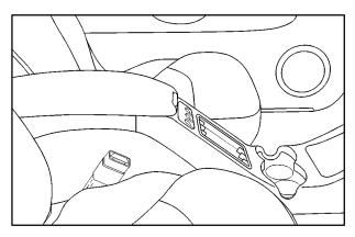
If your vehicle has this console compartment, squeeze the front lever while lifting the top to open it. You can store cassettes and compact discs in the slots in front of the compartment. There is also a lift-out storage tray in the console.
