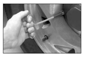
Position the bent end of your hub cap removal tool (shown), or the chisel end of your wheel wrench, in the notch of the hub cap and pry off the hub cap.
