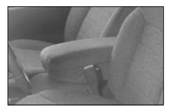
If your vehicle has the center armrest compartment, lift the cover to expose the storage area which includes slots for cassettes or compact discs and a coinholder.
