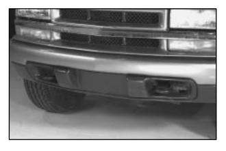
Your vehicle may be equipped with recovery hooks. The hooks are provided at the front of your vehicle. You may need to use them if you're stuck off-road and need to be pulled to some place where you can continue driving.
