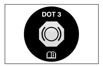
Your brake master cylinder reservoir is filled with DOT-3 brake fluid. See "Engine Compartment Overview" in the Index for the location of the reservoir.
