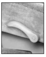
To adjust a manual front seatback, lift the lever on the outboard side of the seat.
