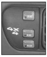
The electronic transfer case buttons are located to the right of the steering wheel.
