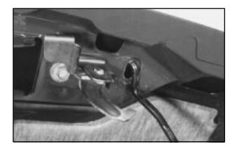
3. Release the hood prop from its retainer and put the hood prop into the slot in the hood
