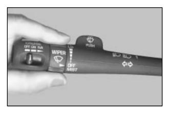
Turn the band with the wiper symbol on it to operate the windshield wipers.
