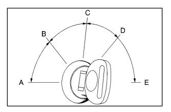
A (ACCESSORY): This position lets you use things like the radio and the windshield wipers and power windows (if equipped) when the engine is off. Push in the key and turn it toward you. Your steering wheel will remain locked, just as it was before you inserted the key.
