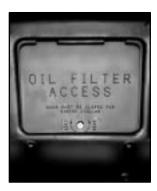
The access door for the remote oil filter is in the steering linkage shield assembly located under the radiator support. Turn the screw to unlock or lock the door. Make sure if you open the door, it is securely closed when you are finished.
