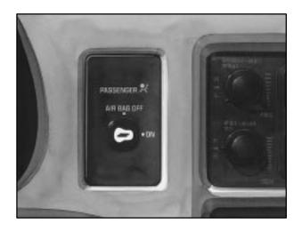
Unless your vehicle has the air bag off switch and the passenger's air bag has been turned off, never put a rear-facing child restraint in the right front passenger's seat. Here's why:
