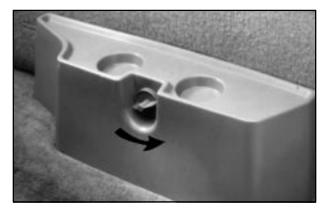
2. Turn the wing nut counterclockwise and remove the wheel blocks, jack and wheel wrench.
