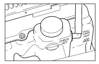
The coolant recovery tank is located toward the front of the engine compartment on the passenger's side of the vehicle. See "Engine Compartment Overview" in the Index for more information on location.
