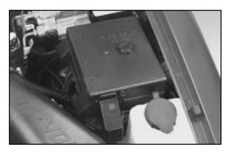
The fuse block is located under the hood on the driver's side of the engine compartment. See "Engine Compartment Overview" in the Index for more information on location.
