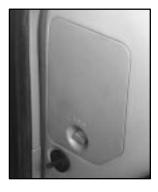
The instrument panel fuse block is located at the end of the instrument panel on the driver's side.
