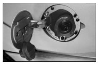
While refueling, hang the cap by the tether from the hook on the fuel filler door.
