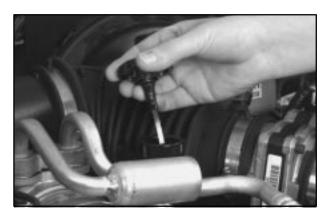
The power steering reservoir is located near the front of the engine compartment on the driver's side of the vehicle.
