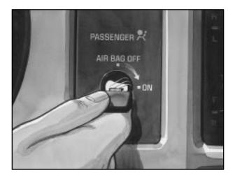
To turn the right front passenger's air bag on again, insert your ignition key into the switch, push in, and move the switch to the on position.
