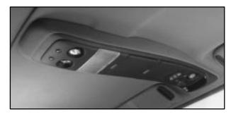
The overhead console includes reading lamps, a compartment for a garage door opener, a temperature and compass display and a storage compartment for sunglasses.
