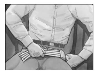
To make it shorter, pull the belt as shown until it is snug. Buckle and position it the same way as the lap part of the driver's safety belt. See "Driver Position" in the Index. Make sure the release button on the buckle is positioned so you would be able to unbuckle the safety belt quickly if you ever had to. To unlatch the belt, just push the button on the buckle.
