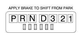
Your automatic transmission has a shift lever on the steering column.
