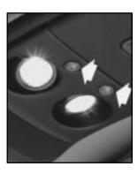
Press the button near each lamp to turn the reading lamps on and off.
