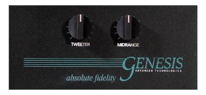
The upper left knob on the back plate marked "**Tweeter**" is a volume control for the front tweeter. Turning this control clockwise will increase the level of the front tweeter. Use this control if you need a bit more treble or to increase the apparent space of the soundstage. Start with this control at the 12 o'clock position. There is about a one dB
