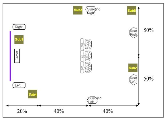
When the third LFE subwoofer is added, place it on one sidewall. If you have a 7.1-channel system, use it to also augment the two right surround and rear channels, and rewire subwoofer #2 to augment the two left surround and rear channels.
