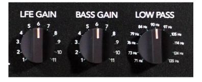
The knob on the middle of the lower row of knobs marked "**Bass Gain**" controls the volume of the built-in bass servo amplifier. Begin with this control at 6 (the 12 o'clock position). Adjusting the gain higher will make the loudspeaker sound "fuller" and more bass-heavy.
