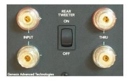
As these speakers are dipolar with a rear-firing tweeter, there should be at least 12 inches (30cm) of space between the back of the speaker and the wall. If this space is not available, switch the rear tweeter off with the tweeter defeat switch.
