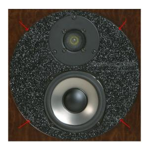
You will notice that the tweeter and midrange drivers are mounted on a round plate secured with four screws. These screws can be removed, and the plate rotated by 45 degrees so that the tweeter and midrange are at an angle, or rotated by 90 degrees so that the tweeter is above the midrange. If you do rotate the midrange and tweeter, it would still be better to have the rear tweeters closest to one another.
