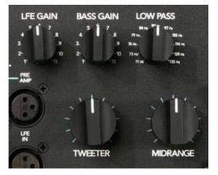
The knob on the upper middle marked "**Bass Gain**" controls the volume of the built-in bass servo amplifier. Begin with this control at position 7. The knob on the upper right marked "**Low Pass**" controls how high the woofer will play. At the extreme low of 71Hz, the woofer will play up to 71Hz, and then begin rolling off, or reducing its volume, above this frequency. The recommended beginning position for this control is 90Hz.
