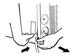
Gently press inward on the right side of the case and pull the lower right side of the grille forward to release from the slot.
