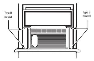
Extend the sliding panels to fill the window opening and use 4 type B screws to secure them, 2 on each side.
