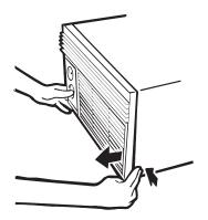
**C** Lift the top of the grille up and off to release from the tabs.
