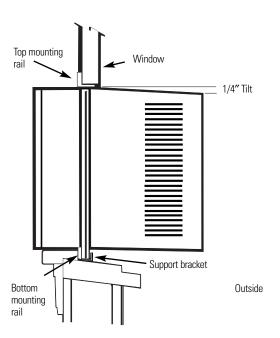
Close the window. Make sure the window sash is behind the top mounting rail of the air conditioner. A 1/4" slant from the front of the case to the rear is necessary. Use a level to determine the slant.
