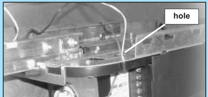
FIG. 1-12 Run wire to power head.
