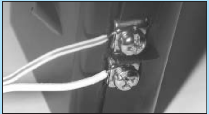
FIG. 3-7 Terminal attachments at STB.
