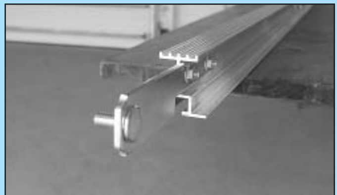
FIG. 1-4 Attach rail strap.
