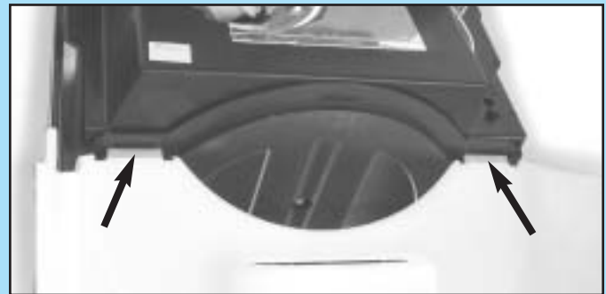
FIG. 10-1 Slide hinges into motor cover.
