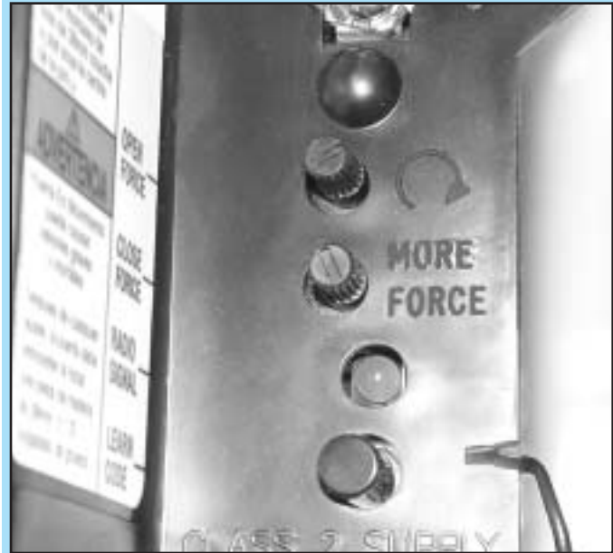
FIG. 7-1 Force adjustment screws.
