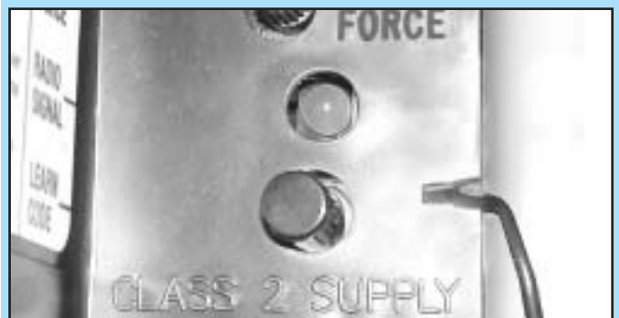
FIG. 8-1 Learn code button and LED
