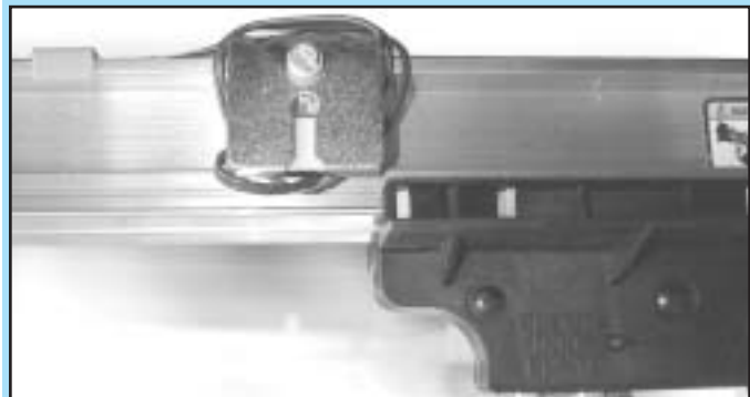
FIG. 7-3 Align “CLOSE” limit switch.
