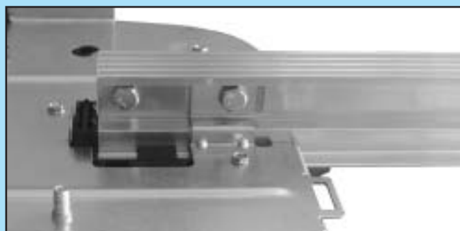
FIG. 1-7 Attach rail to power head.
