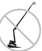
Do not depend on the tilt alarm as a level indicator. The tilt alarm sounds in the platform only when the machine is on a severe slope.
