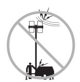
Do not connect wires directly to the generator. Connect auxiliary equipment only to the power outlets provided.
