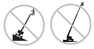
Do not raise or extend the boom unless the machine is on a firm, level surface.
