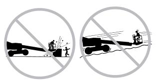
Limit travel speed according to condition of ground surface, congestion, slope, location of personnel and any other factors which may cause collision.
