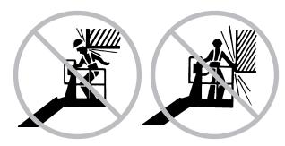
Be aware of crushing hazard when grasping the platform guard rail.
