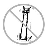
Do not raise the platform unless the base is level, all four outriggers are properly set up and the leveling jacks firmly contact the ground.
