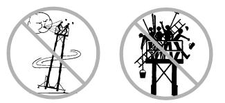
Occupants, equipment and materials shall not exceed the maximum platform capacity.
