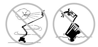
Use extreme care and slow speeds while driving the machine in the stowed position across uneven terrain, debris, unstable or slippery surfaces and near holes and drop-offs. Do not drive the machine on or near uneven terrain, unstable surfaces or other hazardous conditions with the boom raised or extended.
