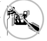
Do not modify or alter an aerial work platform without prior written permission from the manufacturer. Mounting attachments for holding tools or other materials onto the platform, toeboards or guard rail system can increase the weight in the platform and the surface area of the platform or the load.
