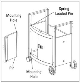
Upper Frame Support , align the mounting hole in the top of the Door and release the spring-loaded pin to secure the Door in place. Repeat this procedure with the left Door.
