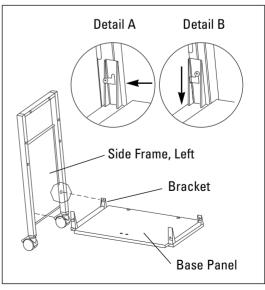
Attach the Base Panel to the right Side Panel, as shown, using three Long Bolts (two may be in panel already), following the same procedure outlined in step 3.
