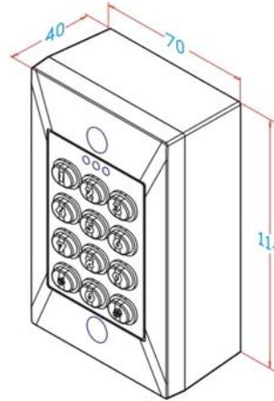
Surface mounting Installation: SMB-750 housing is optional for surface mount.
